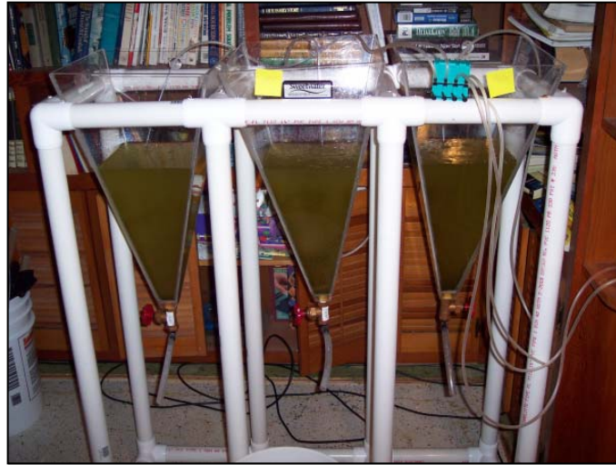
Figure 9. Large 5.5 gallon culture cones used for both brine shrimp and rotifers. Having a drain valve on the bottom of both large and small culture cones is very handy.
