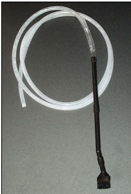
Figure 8. Micro Brush Cleaner used for cleaning bare bottom
